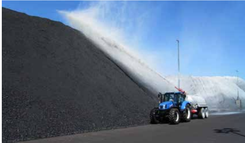
Image 20 A crust of paper-like material is applied to prevent dust being spread around by the wind. The (patented) product consists of pellets made from a mixture of cellulose fibres, which are mixed with water and then sprayed on to the 'dusty' stockpiles from specially-designed lorries. (photo: Den Bakker Bedrijven B.V.)
